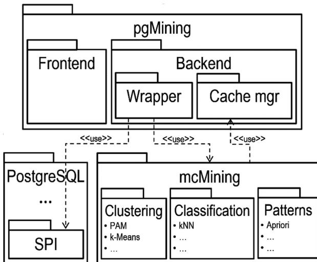
**Fig. 2.** Component structure of the proposed approach
