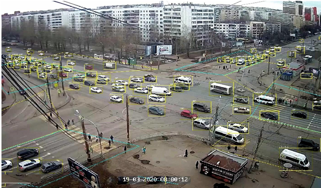
Example of neural network operation for car recognition
