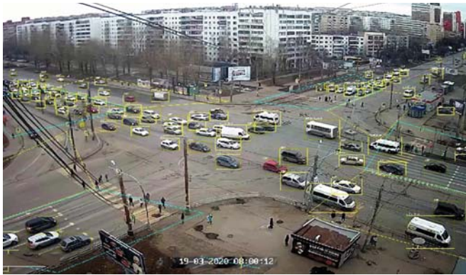
Fig. 4. Example of neural network operation for car recognition
